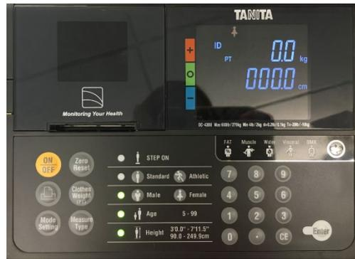
3. “88888 kg” will blink until the machine is ready for use. Then the control box displays “Step On”, prompting for the subject to get on the electrode pads. **The feet should make contact on all 4 electrode surfaces.**
