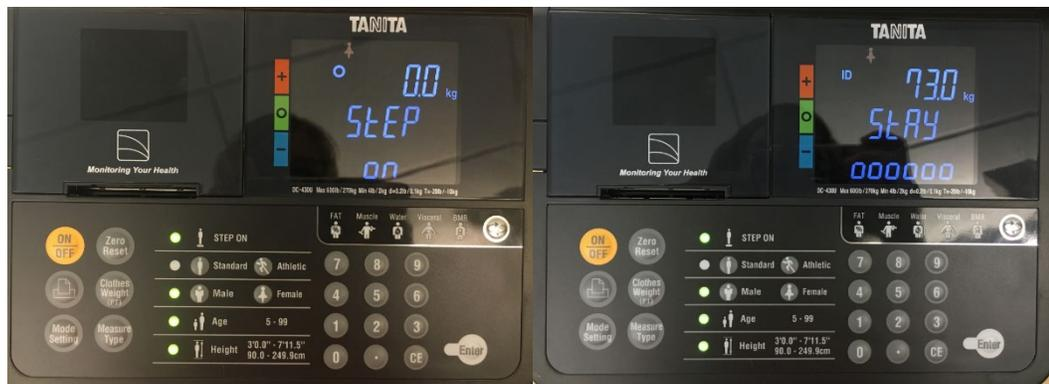
4. The subject will then be measured for the body composition data. The process is complete once there is a beep and the weight in kilograms, kilograms of body fat, and body fat % is displayed on the control box.
